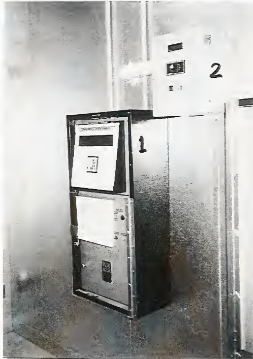
Fig. 3.4 Freezing-and-thawing chamber operating post: 1 - computer; 2 - commutator box with temperature indicator connected to the 12 thermocouples.
