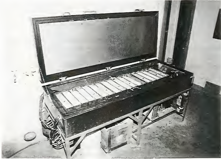
Fig. 4.10 Positioning of 3"x4"x12" specimens in the freezing-and-thawing machine
