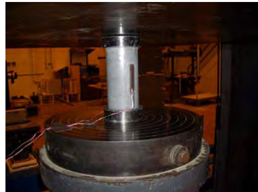
Figure 3.12 Measured stress-strain relationship for HSC and corresponding instrumented cylinder
