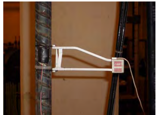
b) Close-up view of a No. 8 tension coupon with an electrical resistance strain gage and a 2-in. gage extensometer
