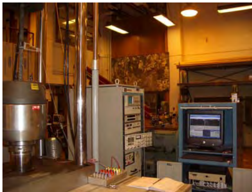
a) Four-pole MTS® testing machine, controller and data acquisition system
