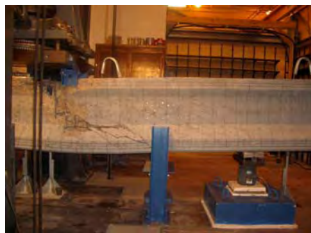
Figure 4.10 Final crack pattern of prestressed concrete specimens
