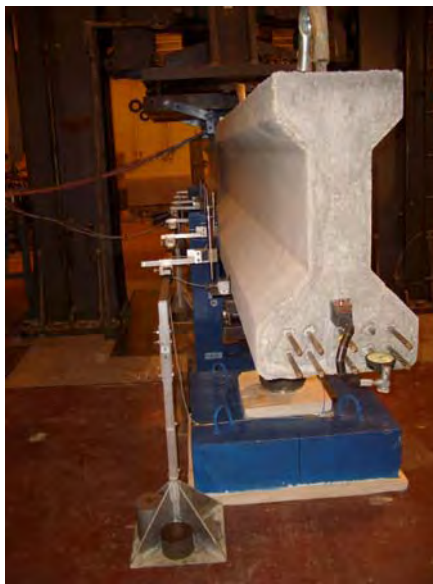
a) Detail of LVDTs, inclinometer and dial gage for relative displacement of prestressing strands
