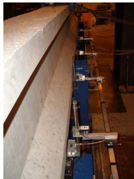
b) Close-up view of LVDT and inclinometer at support
