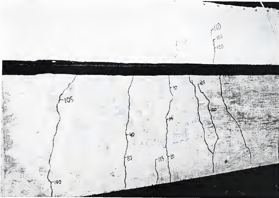
T-Beam FWC-3" Stirrup Spacing (North Face)
