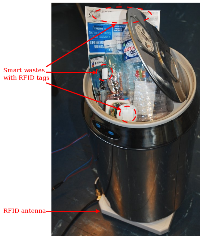
Figure 6. An individual bin using the RFID technology.
