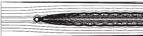
Fig. 27. An instantaneous vorticity field snapshot for \epsilon = 0.01 and B = 0.1 at Re = 3000 and Wi = 6.0 .
