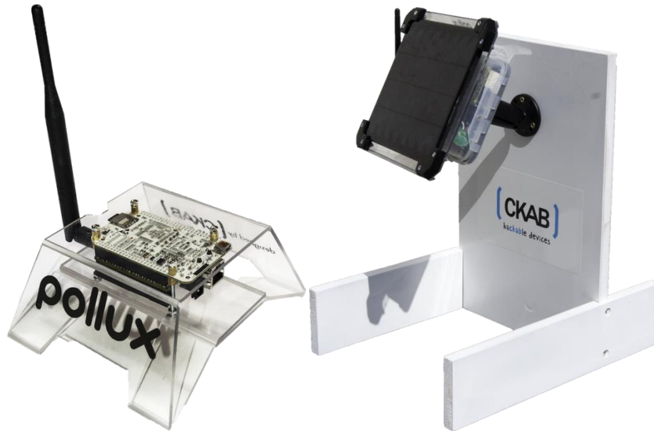
Figure 97: Pollux green station (gateway module and sensors)
