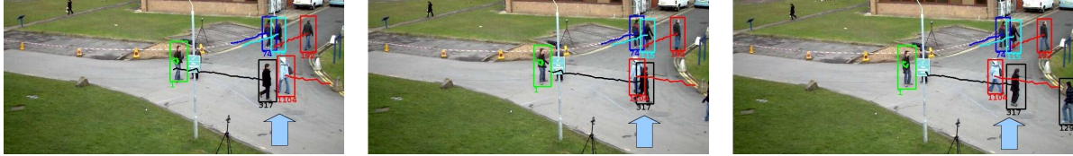
Figure 4. Discriminative Appearance-based tracker: Two persons of Ids 317 and 1104 (marked by the cyan arrow) keep correctly their ids after occlusion as they have very different color appearances.
