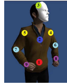
Fig. 2. Virtual avatar used and the position of the nine articulation joints used to animate it.
