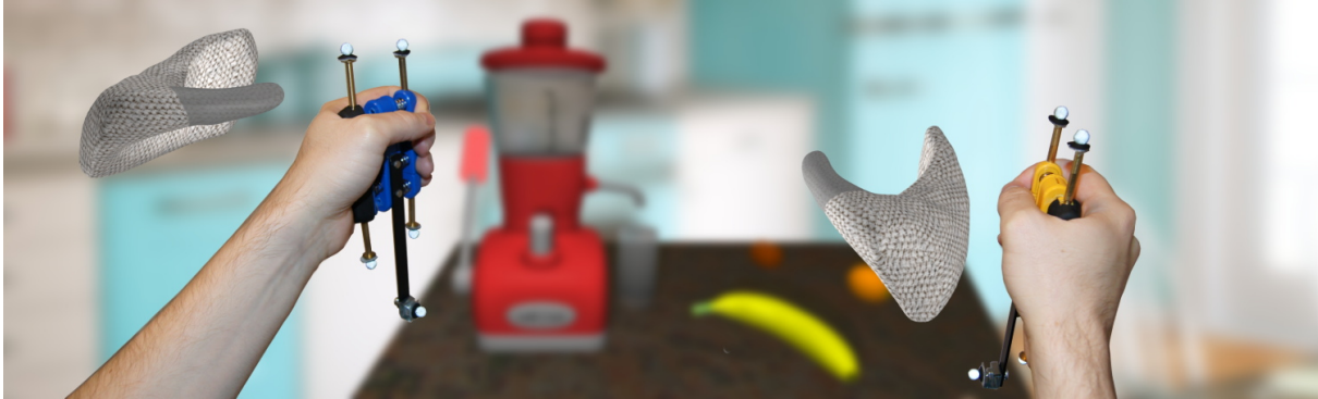
Figure 1: Visuo-haptic manipulation as enabled by our novel approach called the “Virtual Mitten”. Each hand holds an elastic device to control a corresponding virtual mitten (in gray) and to grasp virtual objects in a bimanual scenario. The grip force applied by the user is measured to generate pseudo-haptic feedback.
