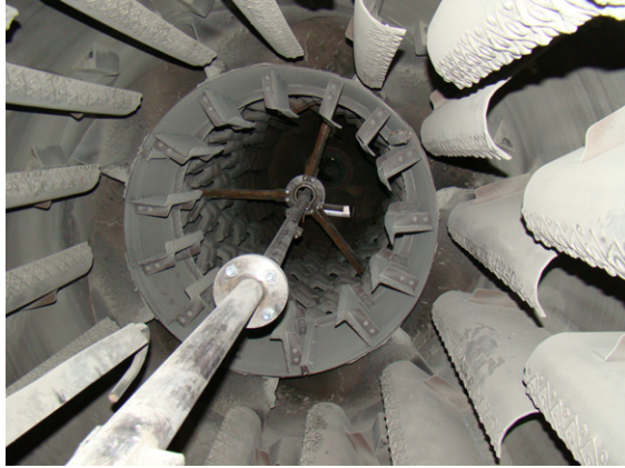
Figure 1 - View of an empty rotary drum used in the Hot-Mix-Asphalt (HMA) plant and equipped with the probes rod.
