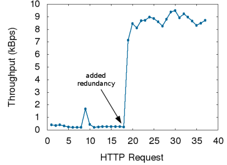
Fig. 6. Throughput before and after handover.
