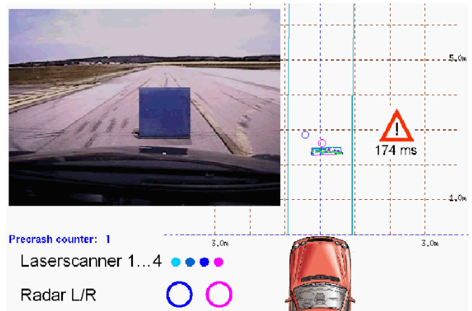
Fig. 2. Visualization of the environment perception on the in-vehicle screen. The inset shows the scene recorded by the camera behind the windshield.
