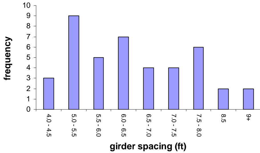
Figure 4.16 Representative Bridge Histogram (Girder Spacing)
