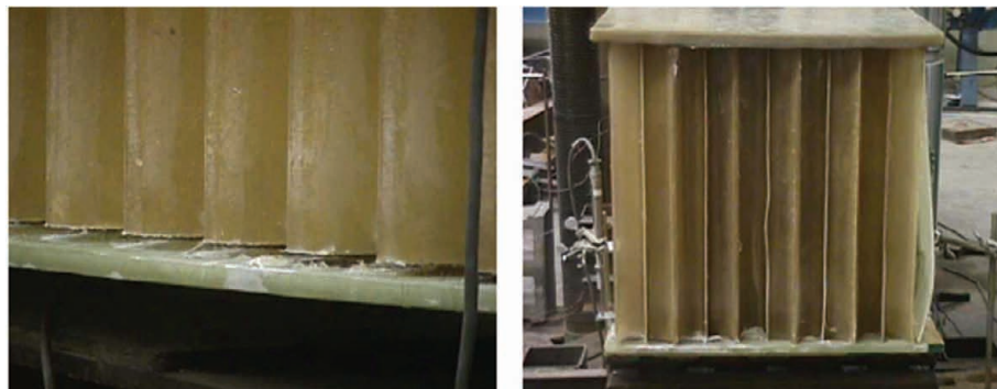
Figure 2.18: Delamination (a) and Buckling of Core (b) for honeycomb sandwich panel (Nystrom, et al., 2002)
