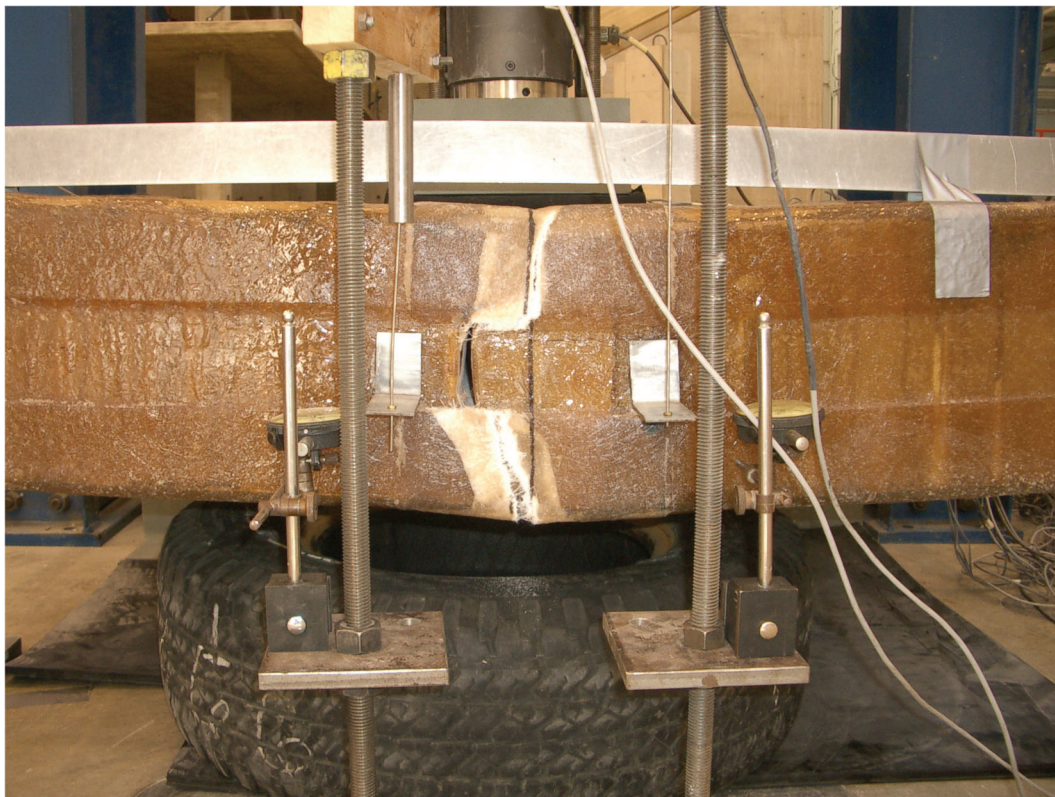
Figure 4.15: View of Longitudinal Joint Damage at Overhang – KSCI #P1a Test
