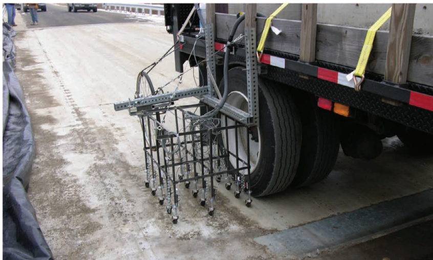
Figure 6.33: Truck with Deflection Frame Attached at Rear Wheel, at End of Path
