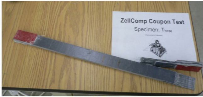
Figure 6.9: Tension Coupon (Fibers Transverse) After Test
