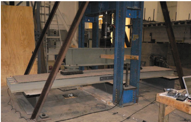
Figure 5.39: Wearing Surface Specimen in Loading Frame
