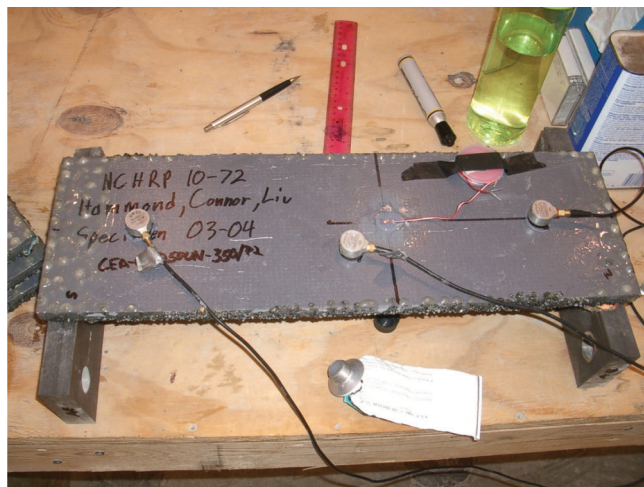
Figure 6.15: NCHRP Wearing Surface Specimen With Acoustic Emission Sensors
