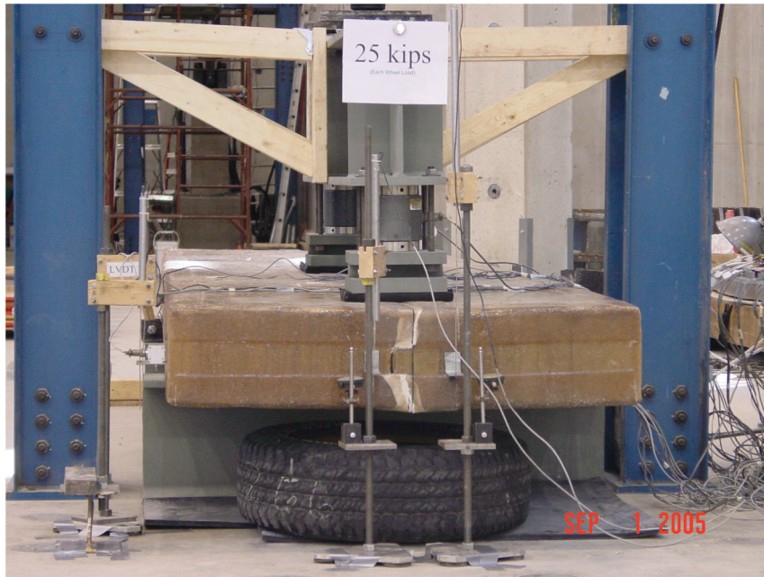
Figure 4.14: Longitudinal Joint Damage at Overhang at 50-kips Total Load – KSCI #P1a Test
