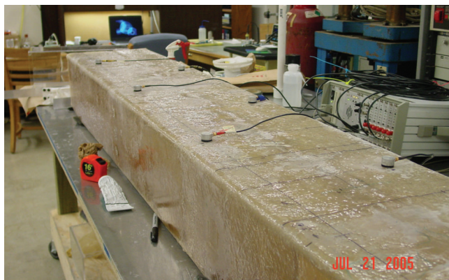
Figure 6.1: Acoustic Emission Sensors on FRP Sandwich Beam for Pencil Test
