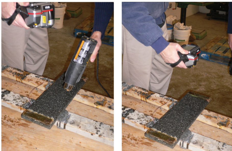
Figure 6.19: Heating Specimen (Left) and Taking Image with Thermographic Camera (Right)
