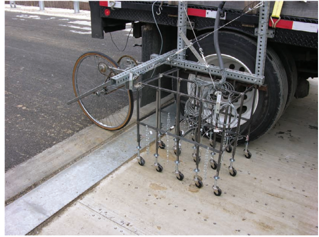
Figure 6.32: Truck with Deflection Frame Attached at Rear Wheel, Stopped at End of Bridge
