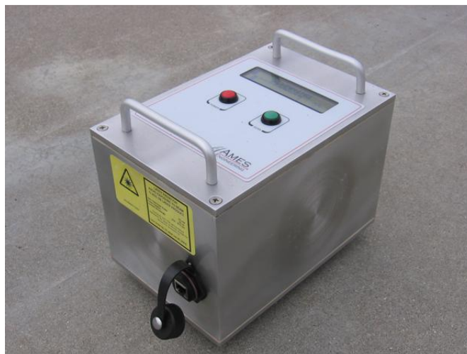
Figure 3-2 The 1 kHz Laser Texture Scanner
