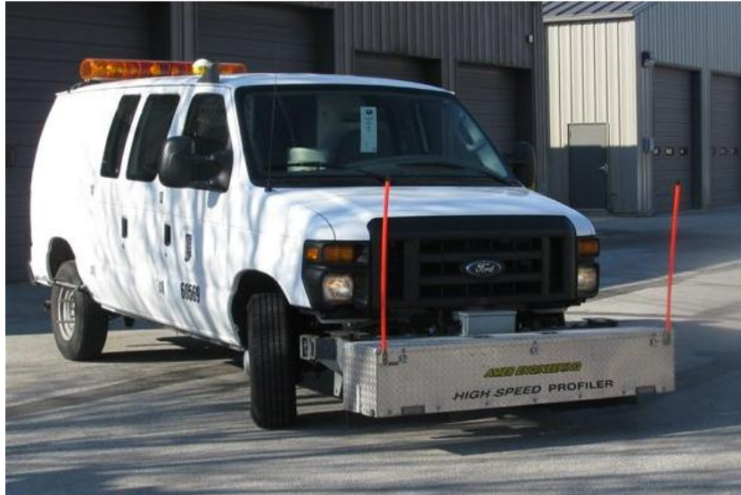
Figure 3-3 The 62.5 kHz Laser System Mounted on a Test Vehicle
