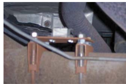
(c) Accelerometer mounted on van axel.
