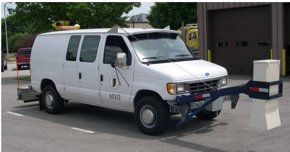
Figure 2: INDOT Laser Profiling Vehicle.
