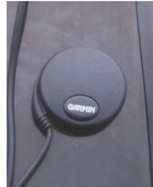
(e) GPS antenna mounted on van roof.
