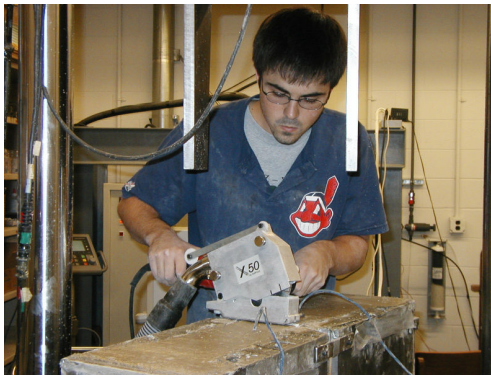
Figure 5.25: Introduction of the saw-cut notch using the early-entry saw
