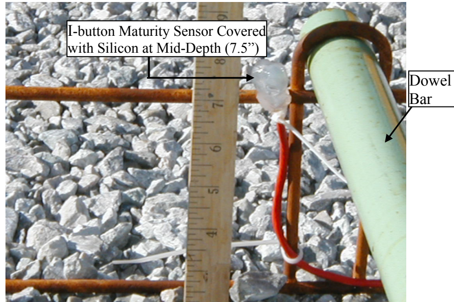
Figure 3.20: Placement of I-button maturity sensor
