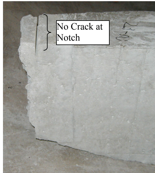
Figure 5.23: Crack propagation for specimen #23 which was cast with a 1.00" (D/8.5") notch and tested at 9 equivalent age hours
