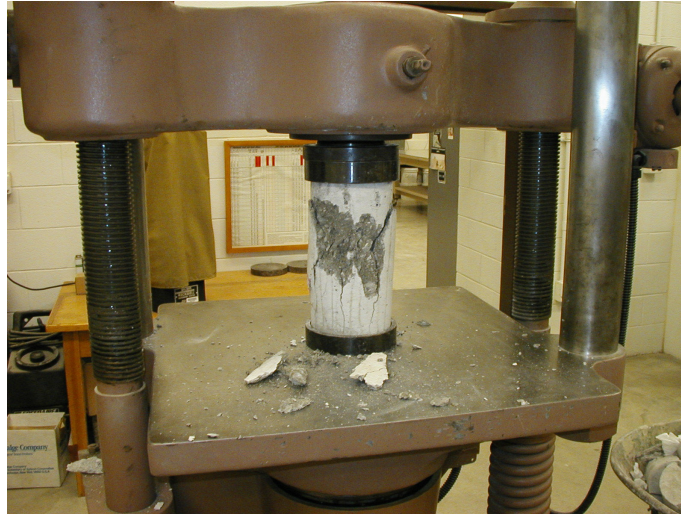
Figure 4.19: 6"x12" cylinder tested in compression at an age of 1 day
