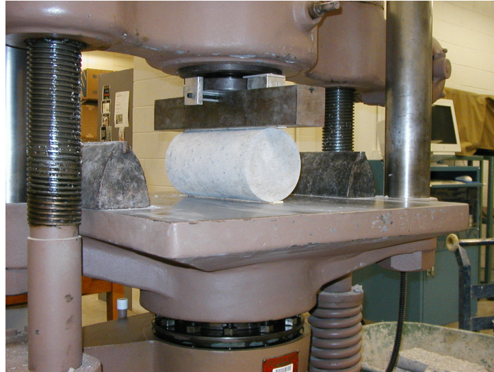
Figure 4.20: Splitting tensile test
