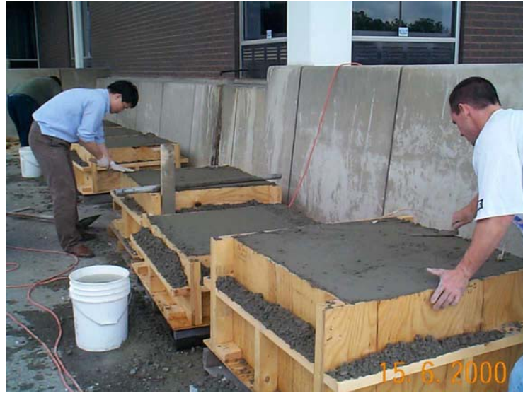
Figure 10-8 Finishing the Surface of the Slabs
