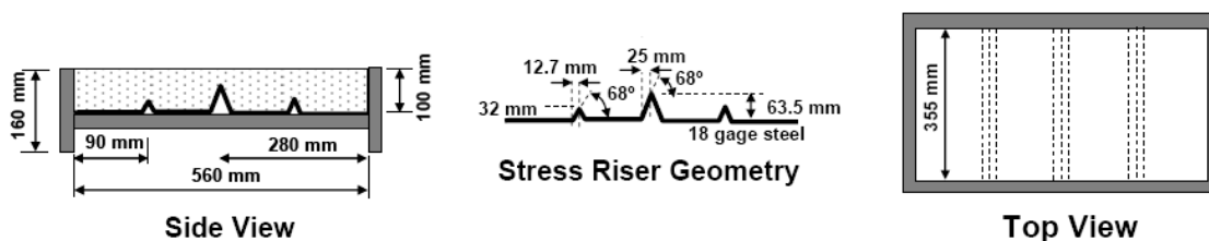
Figure 7-2 – Geometry of the specimens used for plastic shrinkage investigation (Qi et al. 2003b)
