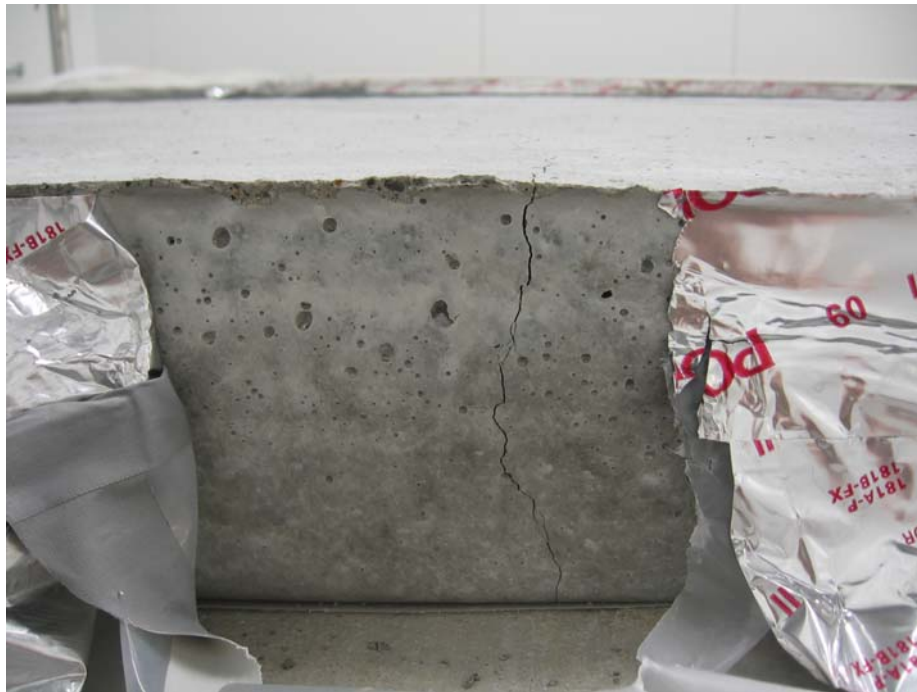
Figure 13-12 – Mixture C-0 Test Slab Crack at 12 Day
