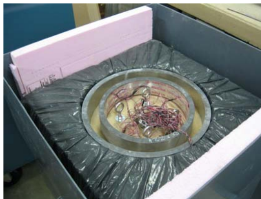
Figure 10-2 - Ring in Insulation Chamber with Top Insulation Removed
