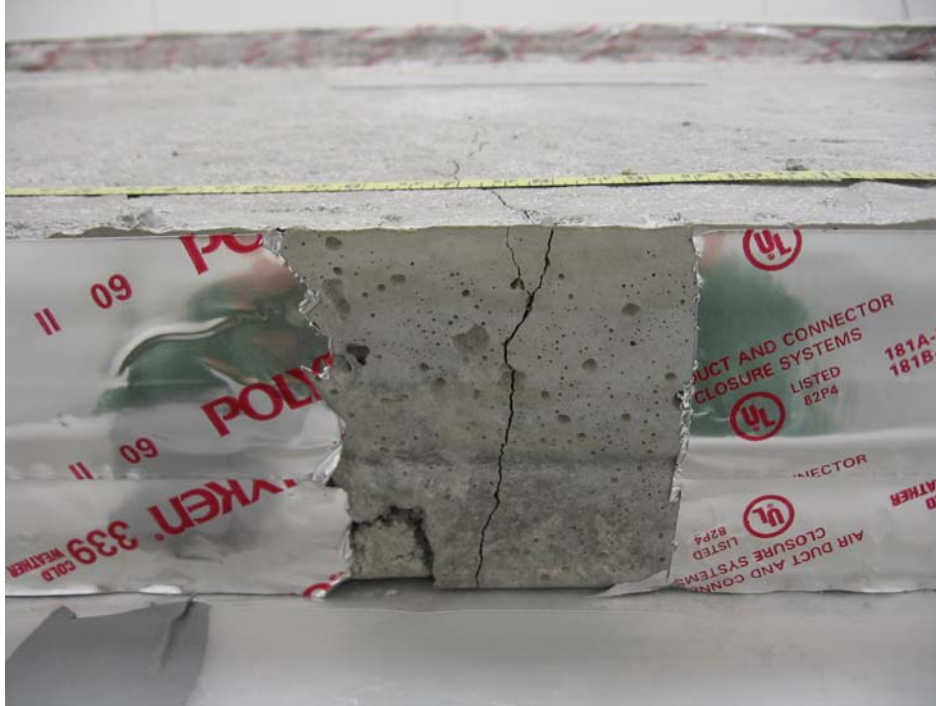
Figure 13-12 – Mixture C-0 Test Slab Crack at 12 Day
