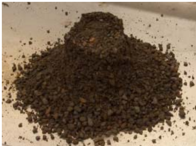
Figure 2-2 – Slight slumping of LWA using the standard cone test in ASTM C128. The slight slumping indicates no surface moisture on the LWA
