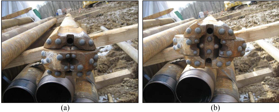
Figure 6.3 A view of (a) folded and (b) expanded drilling bit
