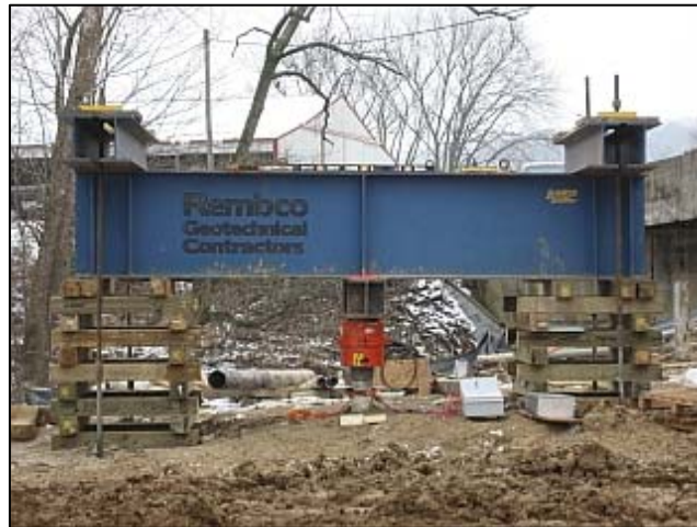
Figure 6.7 Axial load test layout
