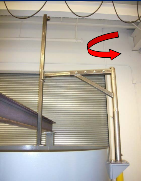
Guide arm for pile driving
