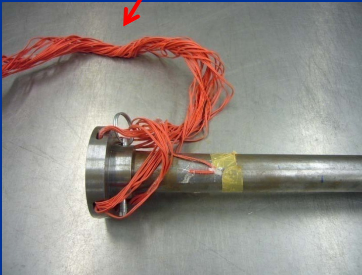
Collected wires at pile head
