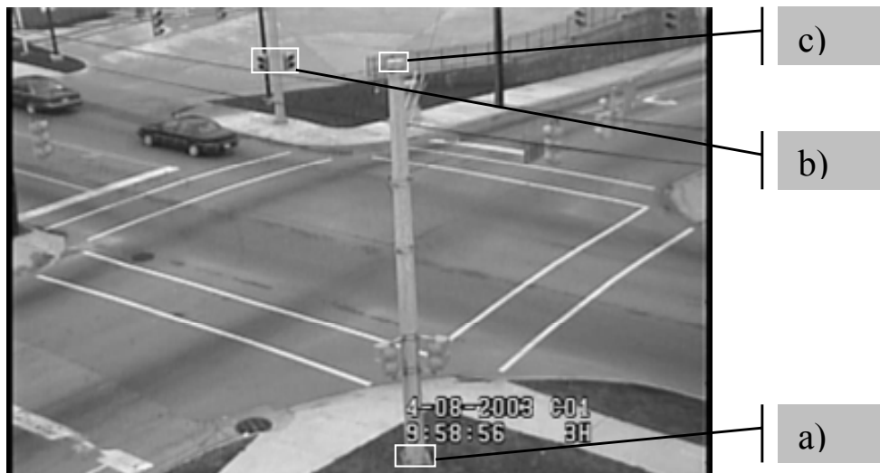
Figure H-13: Locations of the Selected Reference Points for the Vibration Removal Algorithm (97901_10)
