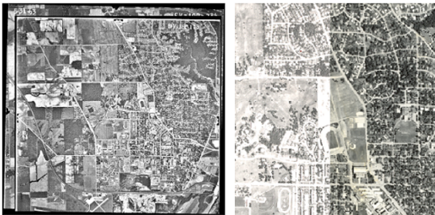
Figure 3. Left: Automatically referenced image (1963) overlaid by reference image (1971), Right: Detailed view of referencing (left light: 1971, right dark: 1963).
