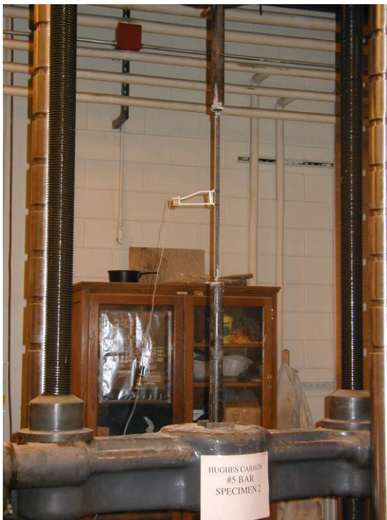
(a) 120 Kip Universal Testing Machine
