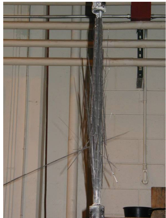
(b) Coupon Test – Carbon FRP (HC1)
