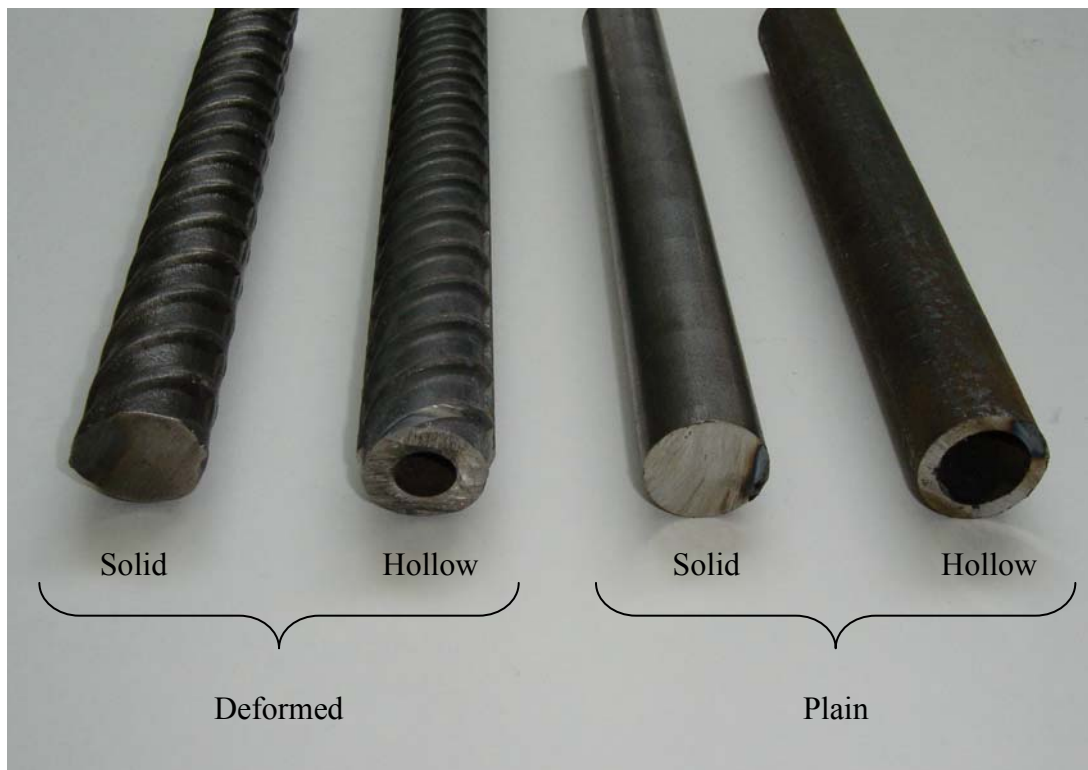
Figure 2.5 Reinforcement Tested to Examine the Effect of Axial Stiffness
