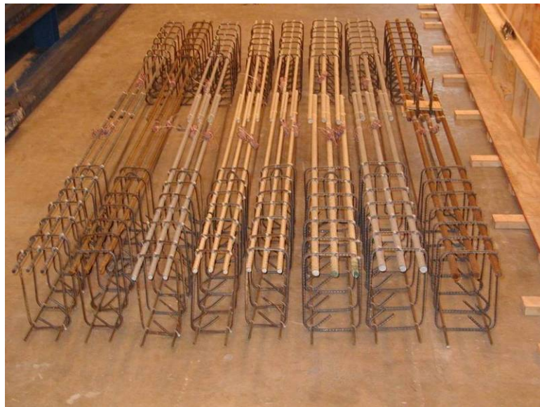
Figure 2.15 Assembled Reinforcing Cage (Series I)
