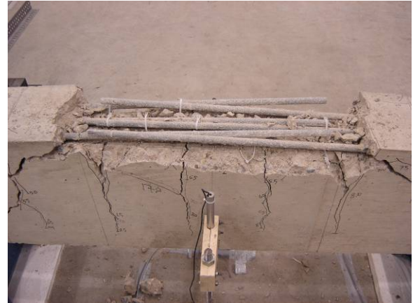
(b) Splice Region after Failure
