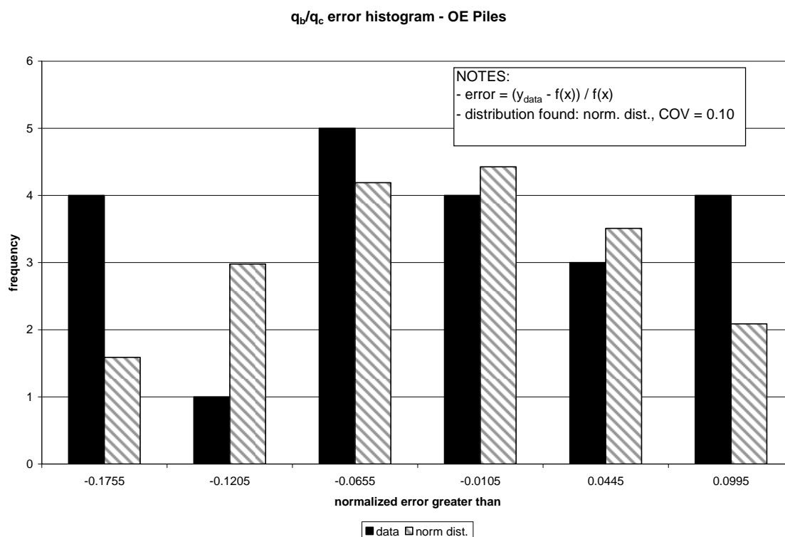
Figure 8.1.12 – Histogram of error_{q_b,10\%/q_c} (detrended q_b,10\%/q_c values) for open-ended piles in sand
