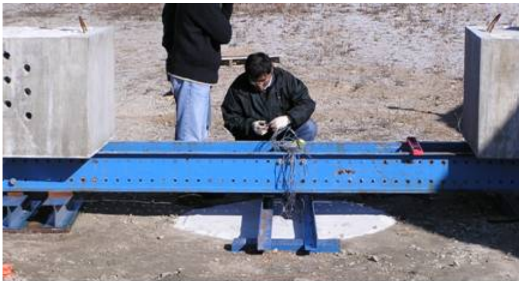
Figure A.12 Reaction beam and counter weights for model pile test
