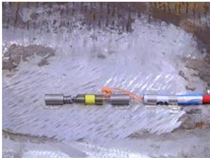
Figure A.2 Spot-welded gage on smoothed pile surface
