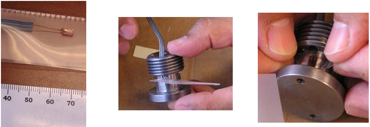
Figure A.7 Electric resistance strain gage attached to the pile base load cell
