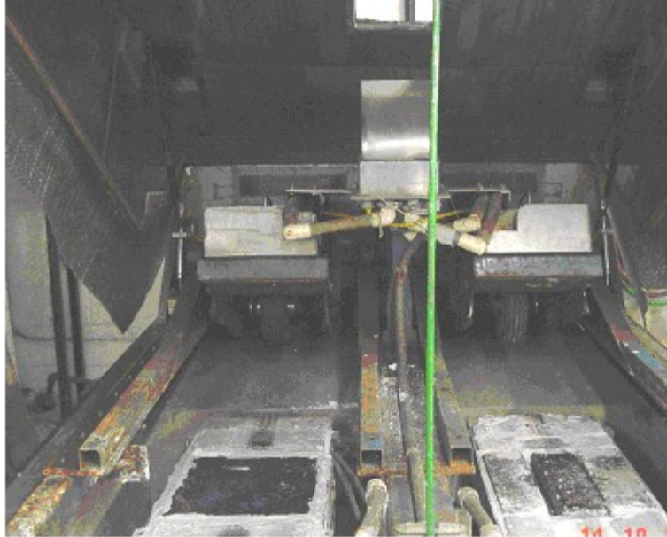
Figure 5.1 Purdue University Laboratory Wheel Tracking Device
