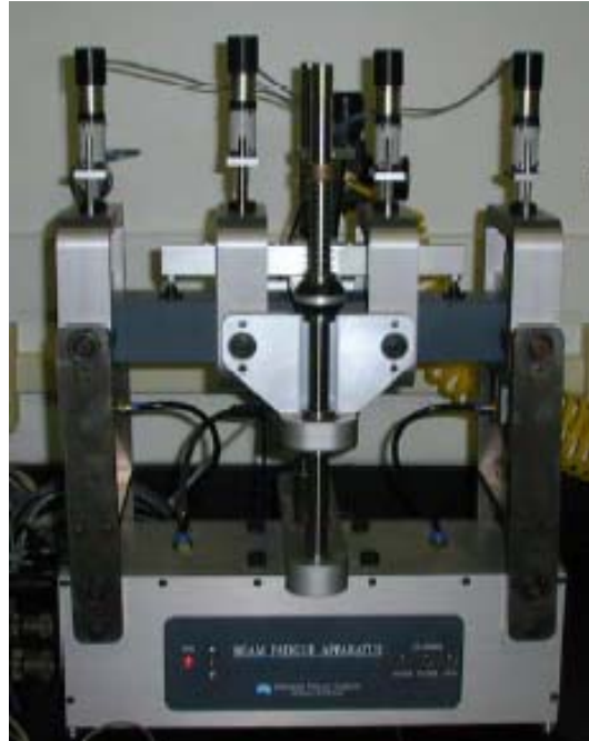
Figure 6.1 Beam Fatigue Test Apparatus
