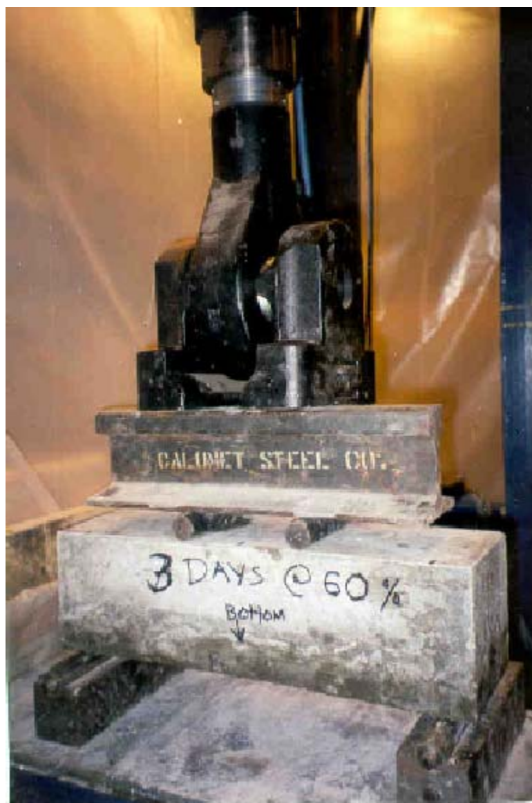
Fig. 7.10 Actuator head touching the loading assembly at the start of test
