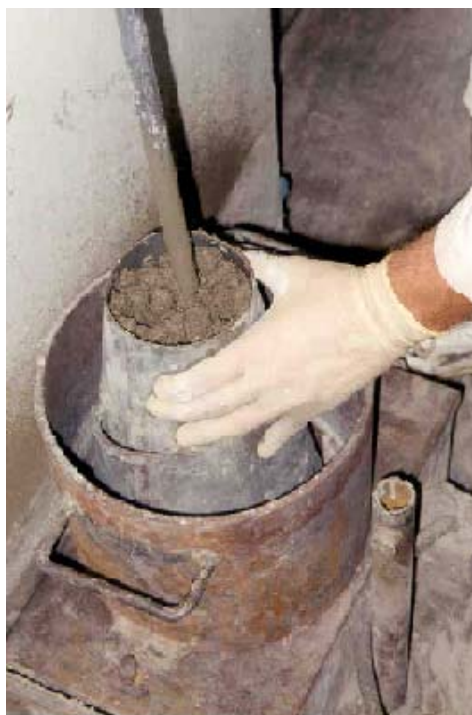
Fig. 7.3 Ve-Be cone top layer being filled
