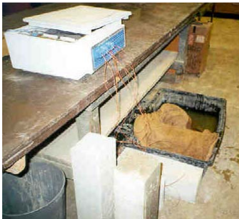
Fig. 8.1 Temperature in specimens being monitored by data-logger
