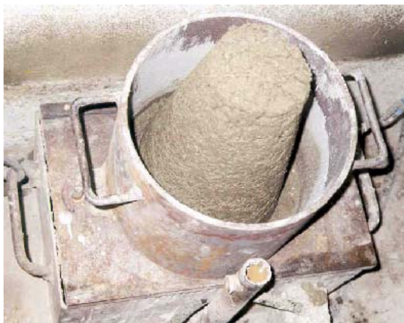
Fig. 7.4 Concrete specimen placed in the test mold on vibrating table right before starting the vibration
