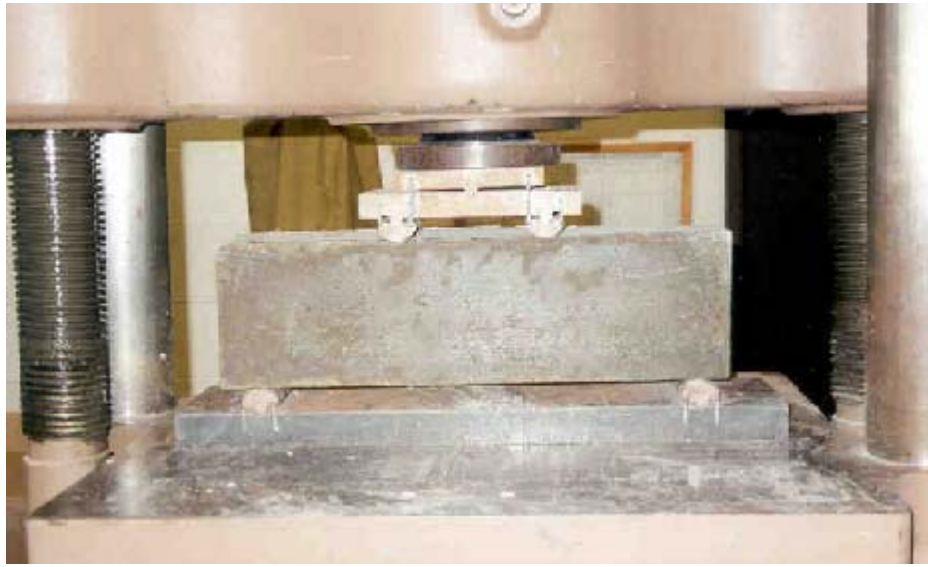
Fig. 7.6 Picture of a 6" x 6" x 12" beam in the testing machine
