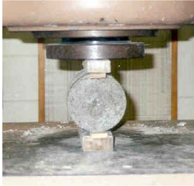
Fig. 7.7 Test specimen loaded in indirect tension
