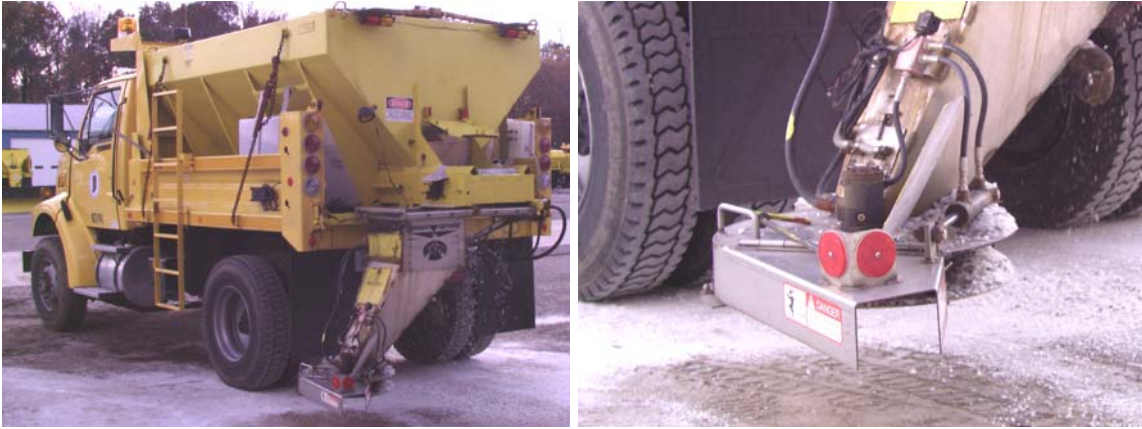
Figure 20 – Swenson Zero Velocity System Figure 21 – Dispensing Unit (Shroud)
