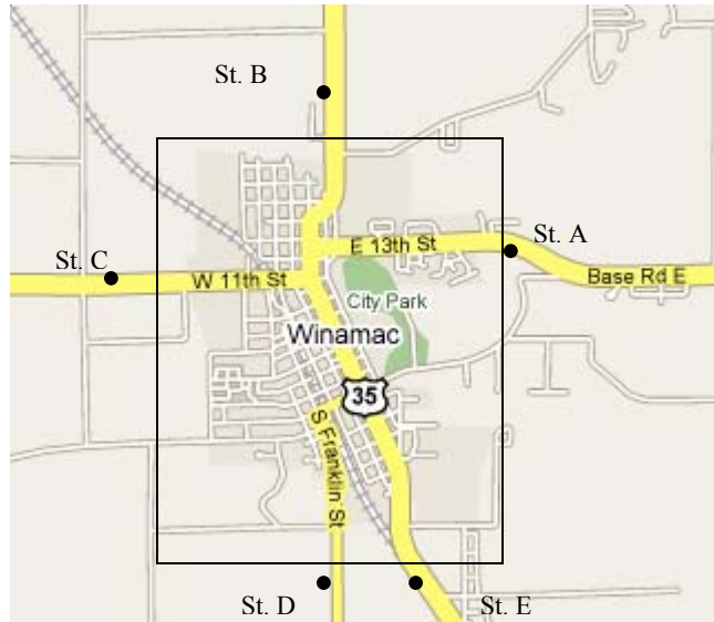
Figure 1.1- Cordon line and external stations for Winamac city
