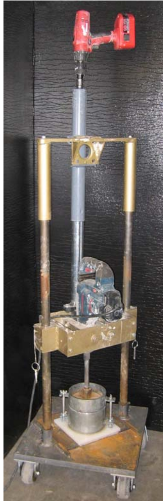
Figure 3.6 Vibrating Hammer modified with mechanical lifting mechanism
