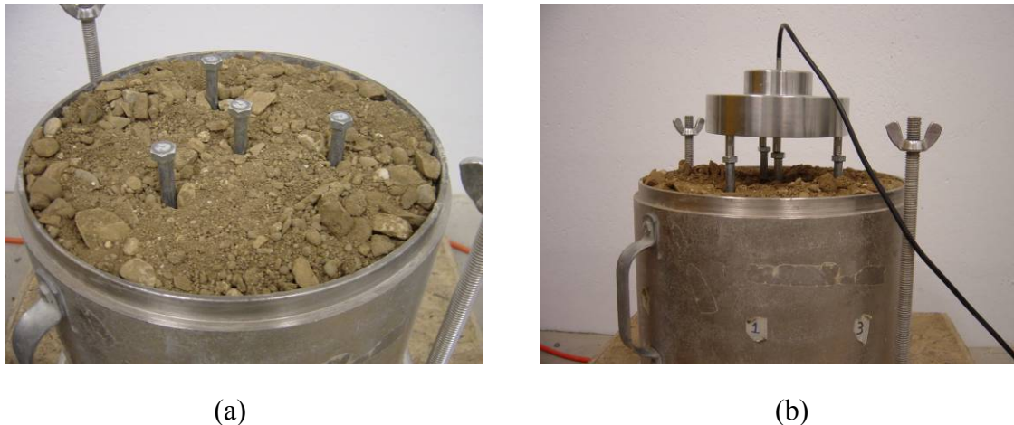
Figure 5.3 TDR testing in 11-inch compaction mold with MRP configuration: a) all conductor rods installed, b) coaxial probe head placed upon conductor rods
