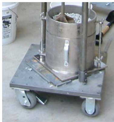
Figure 3.7 Vibrating Hammer modified with heavy duty casters
