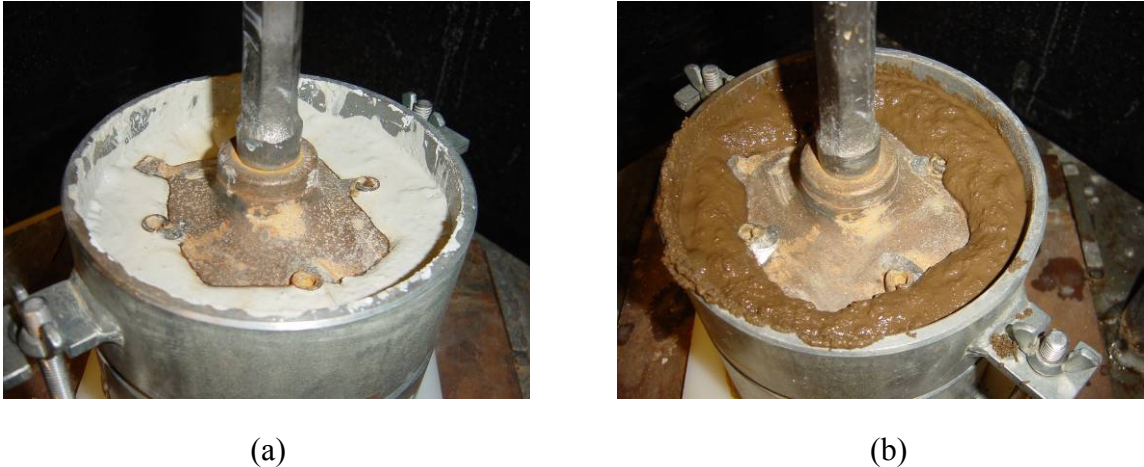
Figure 3.11 Upward fine migration for 6-mold compaction tests near saturation: a) Indiana 53 crushed stone and b) Indiana 53 gravel
