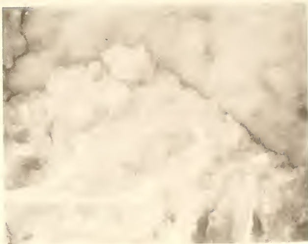
Figure 4.6.7 SEM Micrograph of Mortar From LPF Concrete, w:c = 0.26, at 28 Days (2000X)
