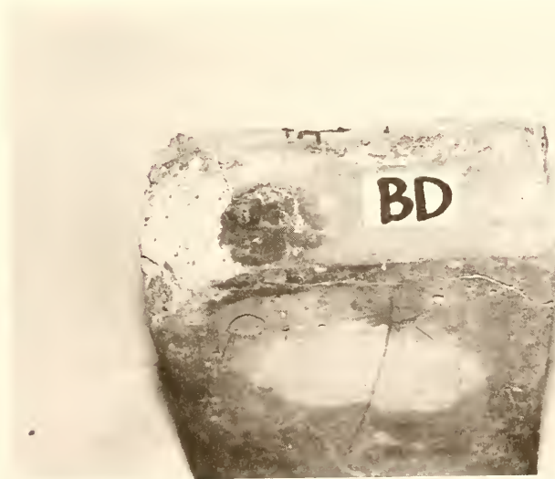
Figure 6.3.2 Close-Up Picture of Damaged BD Concrete Specimen
