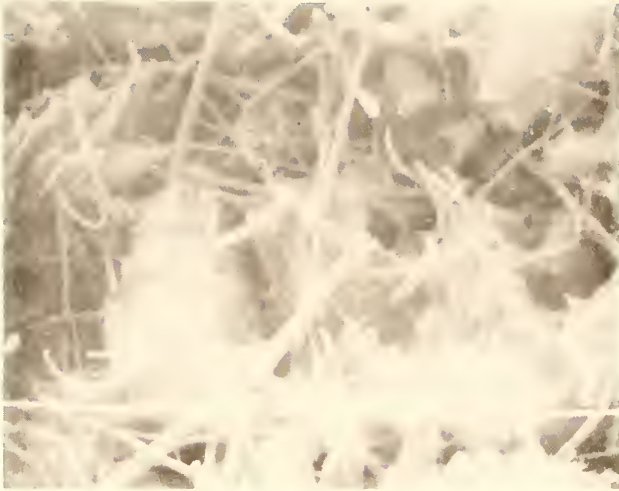
Figure 4.6.17 SEM Micrograph of Mortar from LPN Concrete, w:c = 0.28, at 1 Year (10,000X)
