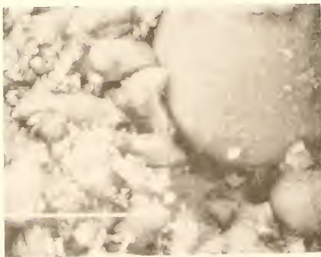
Figure 4.6.8 SEM Micrograph of Mortar From LPN Concrete, w:c = 0.26, at 28 Days (2000X)
