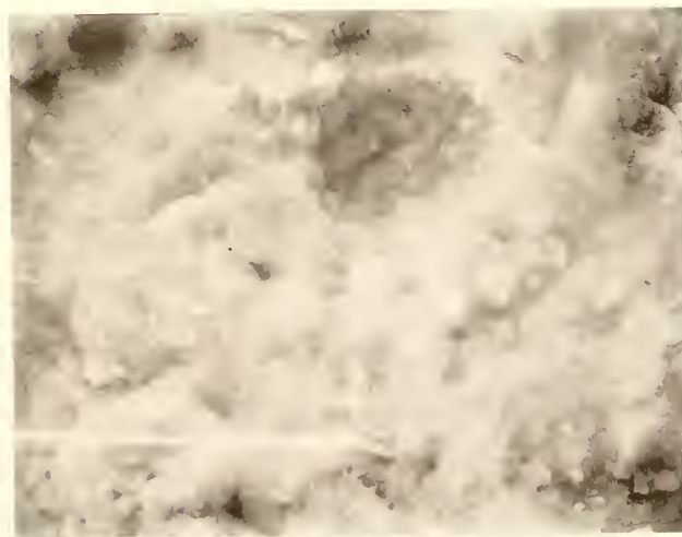
Figure 4.6.6 SEM Micrograph of Mortar From LPF Concrete, w:c = 0.26, at 28 Days (2000X)
