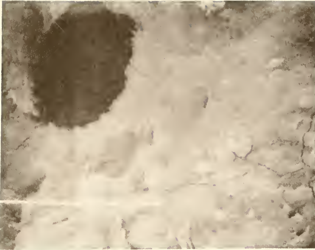
Figure 4.6.13 SEM Micrograph of Mortar From LPF Concrete, w:c = 0.26 , at 1 Year (2000X)
