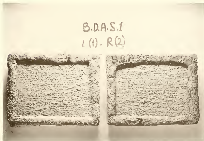
Figure 5.3.2 Appearance of Surface of Air-Entrained BD Concrete After Scaling Test
