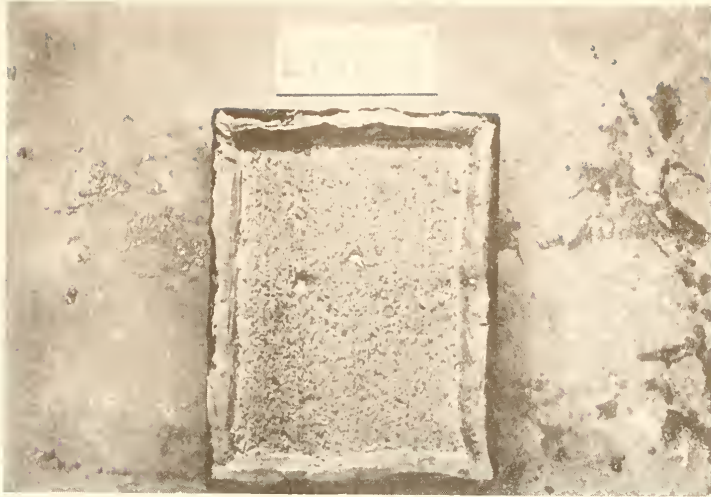
Figure 5.3.7 Appearance of Surface of LPNS-4 Specimens at the End of Scaling Test
