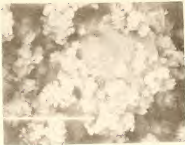
Figure 3.5.3 SEM Micrograph of Fly Ash-CaO Paste, w:s = 0.5, at 3 Days (1500X)
