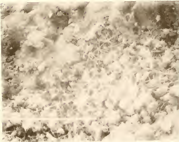
Figure 4.6.16 SEM Micrograph of Mortar from LPN Concrete, w:c = 0.28, at 1 Year (2000X)
