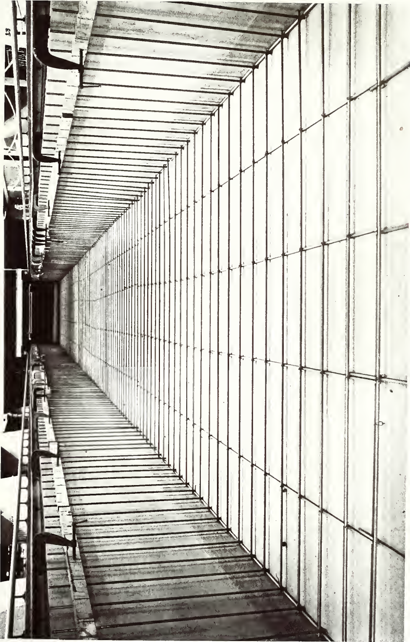
FIGURE 5 - 14 TESTING FLUME WITH ARTIFICIAL ROUGHNESS.
