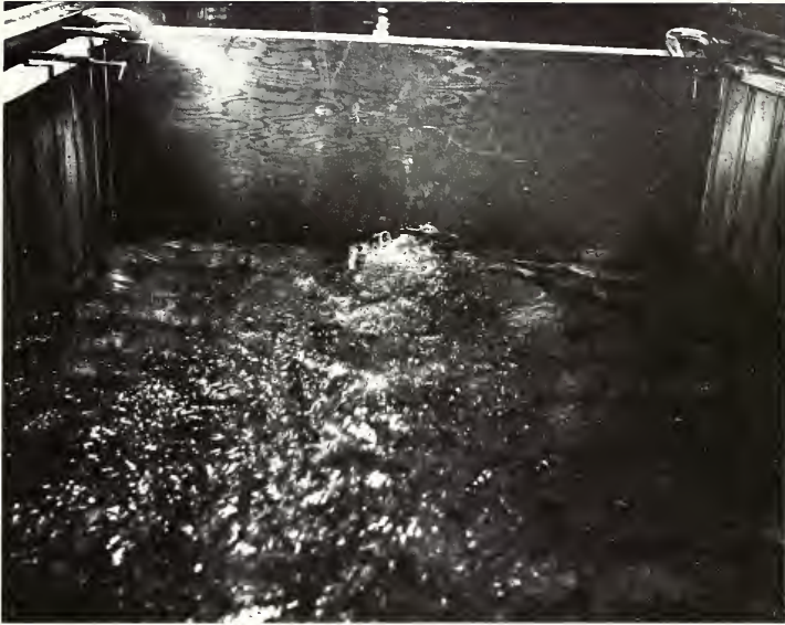
FIG 8-5-3 SLUG FLOW AT BARREL EXIT
