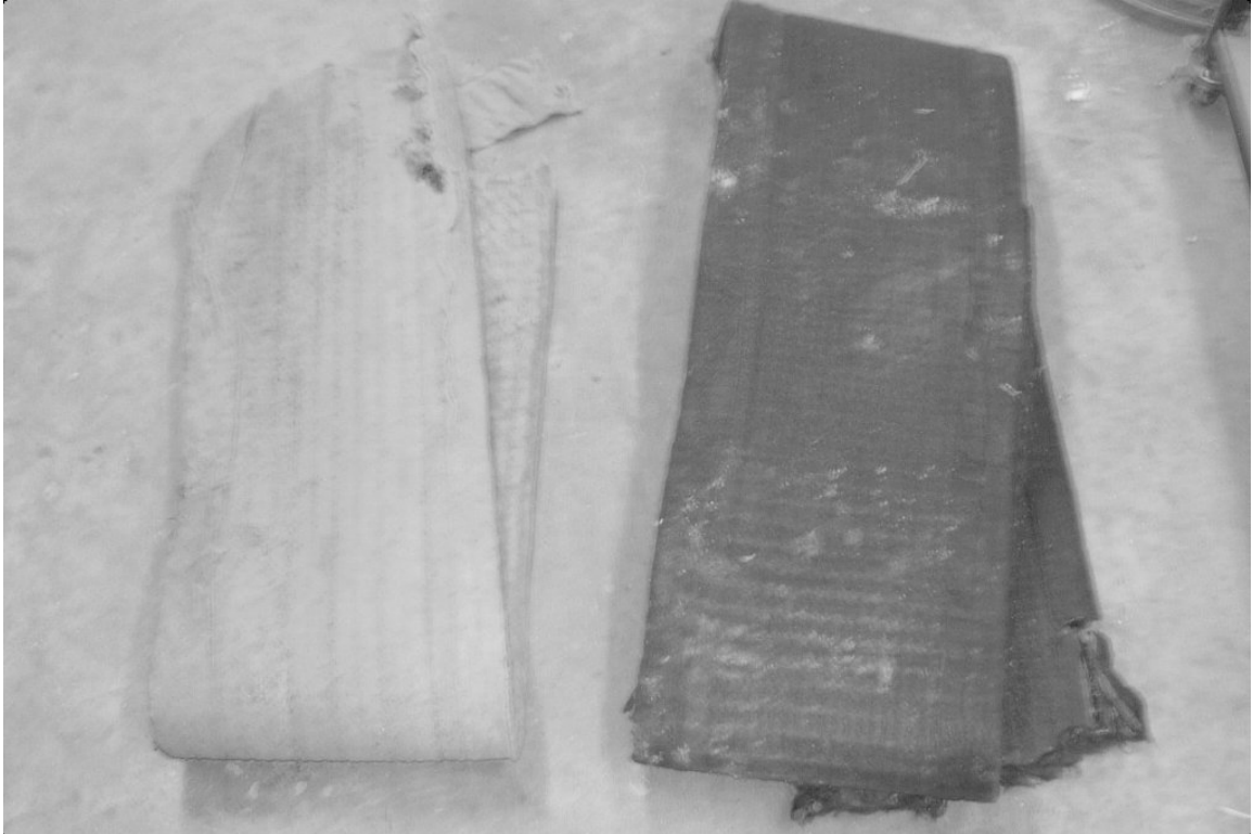
Figure 3-4 Two samples of the same geotextile filter from the Sullivan Co. US 41 site exhumed after 15 years of service: heavily clogged (left-hand side) and almost intact (right-hand side)
