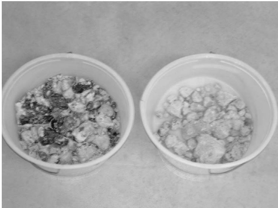
Figure 3-5 Rubbleized concrete aggregates after crushing (LHS : with stabilizer, RHS : after stabilizer is removed)
