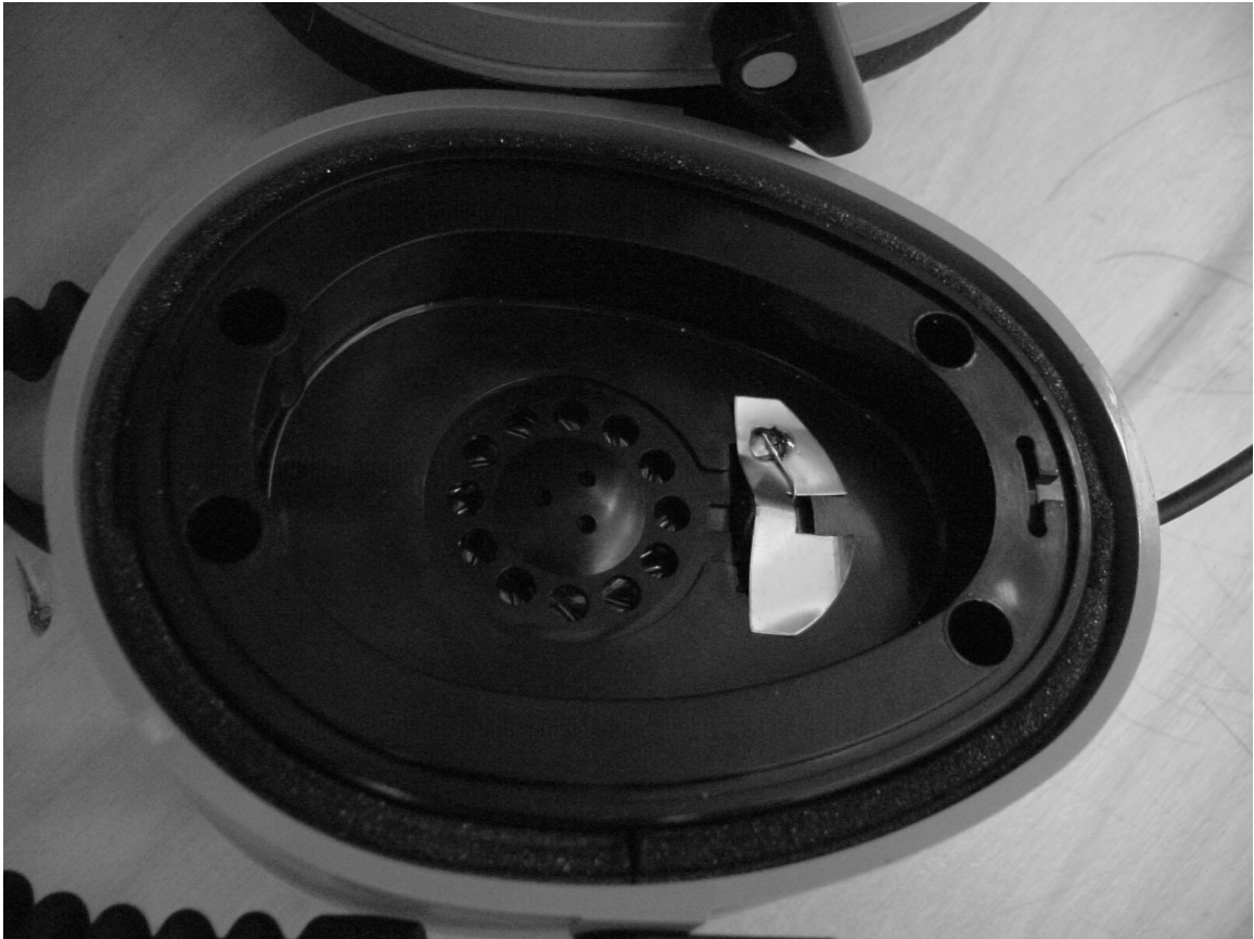
Figure 2.6: Photo of error microphone and secondary source on an exposed ANC headset.
