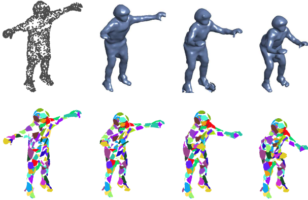
Figure 4. 3D point registration using the proposed approach: ( top ) the implicit interfaces describing different frames 44, 49, 55, 75; ( bottom ) the deformed source patches.
