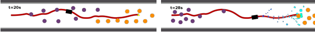
Fig. 3. Navigation using RiskRRT motion planning. The motion prediction uncertainty allied with the high density of agents produces the Freezing Robot Problem, where the algorithm predicts a collision for any possible motion, bringing the robot to a halt.
