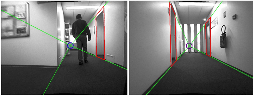
Figure 6: Door detection framework
