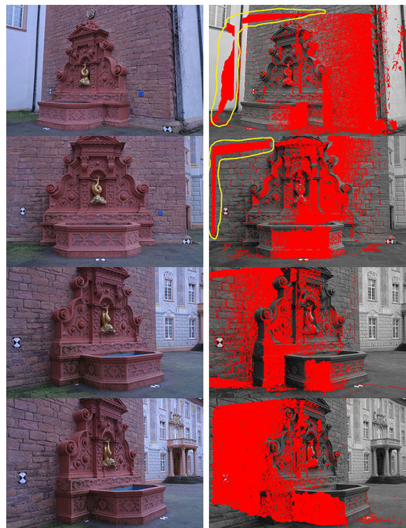
Figure 10. Processing best viewed regions in the Fountain data set [5]. Each view represents the central image of a triplet (other two images not shown). The red-colored regions represent areas best viewed in the triplet. Yellow regions represent regions that are only visible in the triplet and therefore are included even if they do not comply with the best view requirement.
