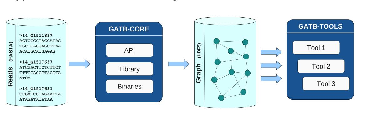
GATB-CORE transforms the reads into a de Bruijn graph, saves it in a HDF5 file that can be opened by other tools developed with the GATB-CORE API.
