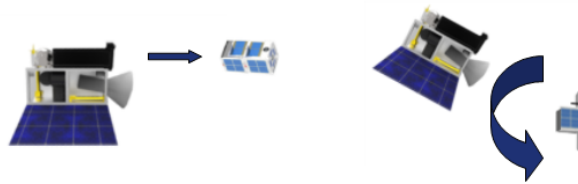
Fig. 3: VBN Experiment . This figure shows the sequence in the VBN experiment: (a) cubesat ejection, (b) VBN manoeuvres.
