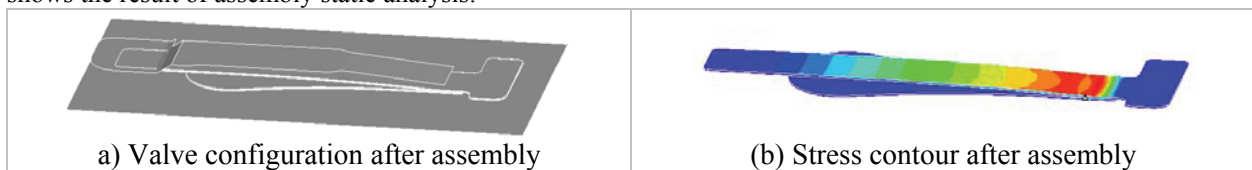
Figure 6: Result of structural analysis of assembly
