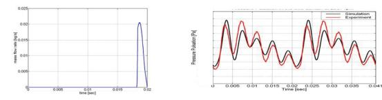
Figure 3. Estimated mass flow rate
