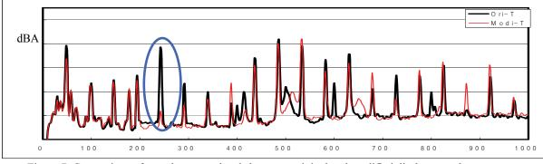
Figure 7. Comparison of sound pressure levels between original and modified discharge paths
