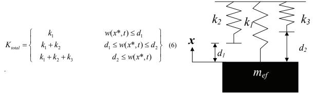
Figure 1. Simplified valve model
