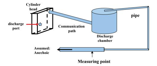
Figure 2. Simplified discharge path
