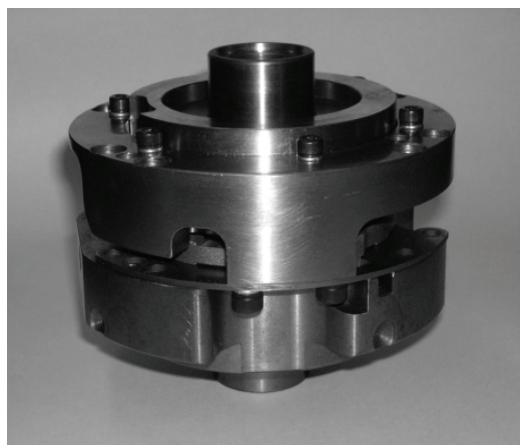
Figure6. Prototype of axial compliance mechanism
