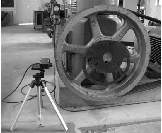
Figure 4 Instantaneous swept volume sensor installation
