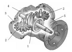
Fig. 1 Basic components of a typical single screw compressor (1-screw rotor, 2- star-wheel, 3-support portion, 4-screw groove, 5-houseing case)
