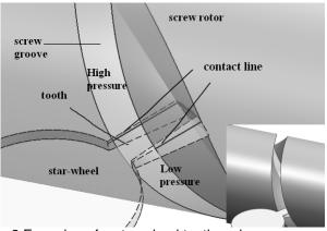
Fig. 2 Engaging of a star-wheel tooth and a screw groove
