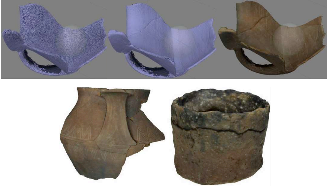
Figure 4. Raw mesh (top left) / smoothed mesh (top middle) / mesh with colors (top right) / textured meshes (bottom)
