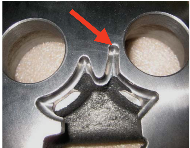
Figure 2: The discharge port of a bus A/C screw compressor, the red arrow indicates important area for drainage of oil
