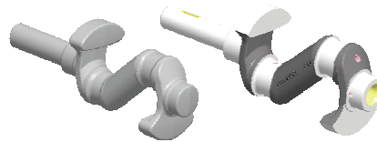
Figure 8.3: Final modified crankshaft.
