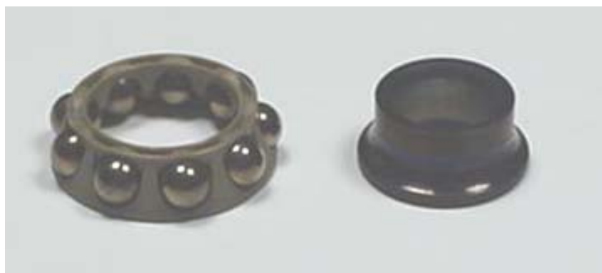
Figure 8: Bearing exposed to extreme heat and air
