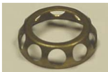
Figure 4: Pressed (stamped) brass cage
